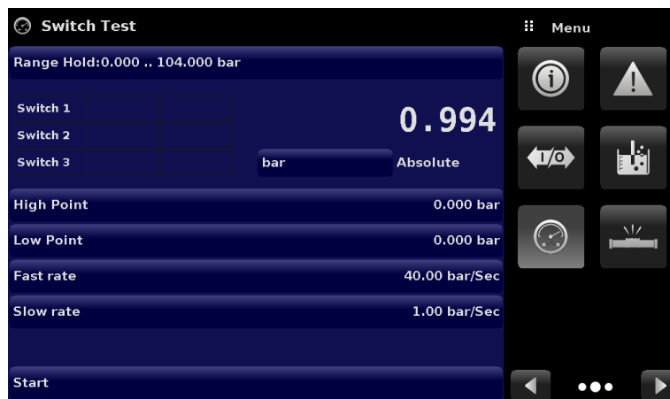
Figure 6.4.13 Switch Test App
