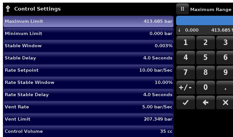
Figure 6.4.3.1 Control limit setting
