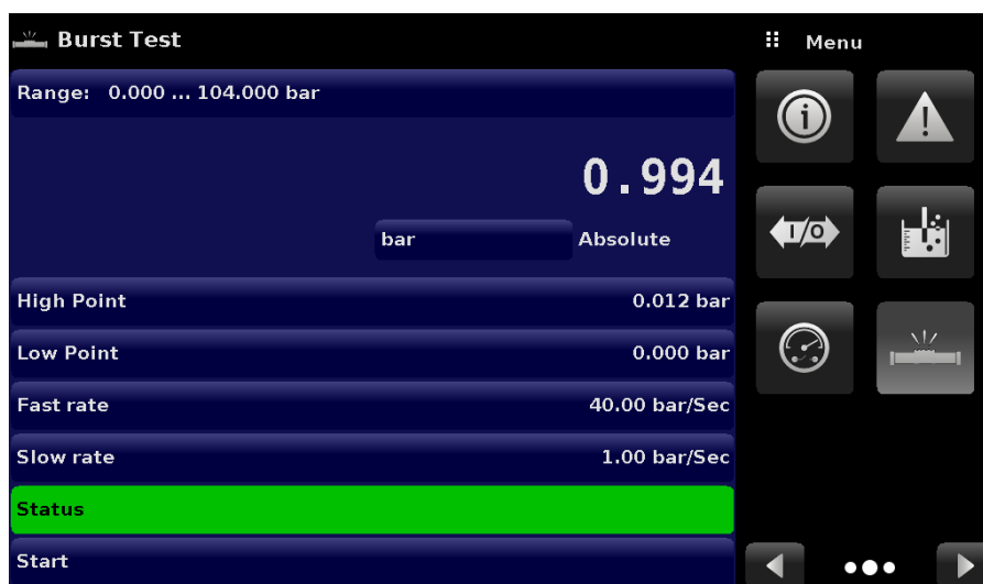
Figure 6.4.14-B Burst Test Complete (No Burst)
